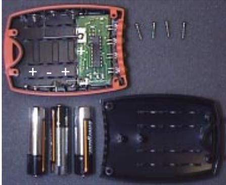
1. On the side opposite the switches, remove the four screws with a small point (#1) phillips screwdriver.
